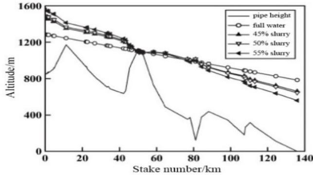
Figure 2. Pressure change diagram of full water and full slurry pipeline transportation
