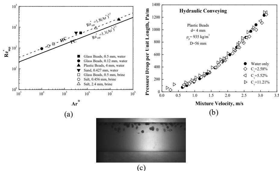
Figure 3. (a) Models for minimum pressure velocity in PC and HC; (b) Phase diagram for plastic beads in HC; and (c) flow visualization.
