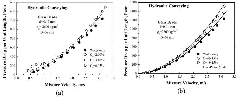
Figure 4. HC of glass beads of (a) 0.12 mm size showing settling behaviour; and (b) 0.01 mm size showing non-settling behaviour.
