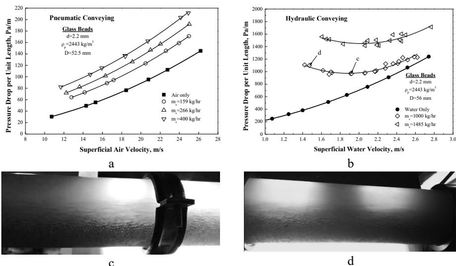
Figure 2. Phase diagrams for glass beads having median size of 2.2 mm in a. PC; and b. HC. Visualizations for flows marked in Figure 2b at c. minimum pressure velocity with sliding bed; and d. the dense phase zone with stationary bed.
