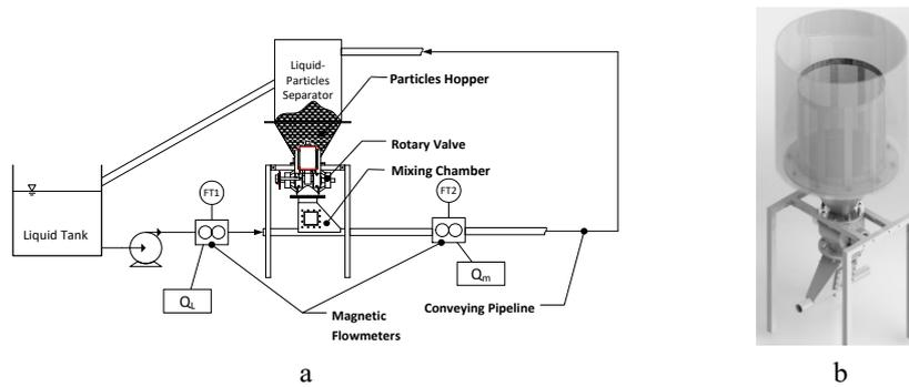
Figure 1. Layout of the feeding zone for the new HC system: a. All feeding devices; b. Separator.
