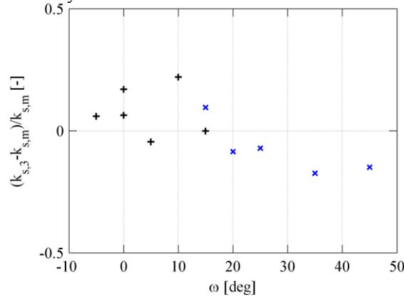
Figure 5. Relative deviation of bed roughness predicted by Equation 3 ( $k_{s,3}$ ) from bed roughness obtained by experiment ( $k_{s,m}$ ). Legend: + – flow at  $V_m = 1.5$  m/s, x – flow at  $V_m = 1.0$  m/s.
