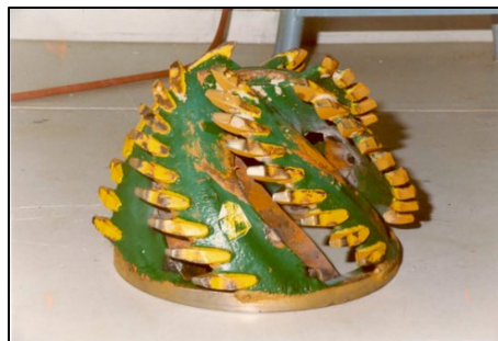
Figure 4. The crown cutter head used by Miltenburg (1982).
