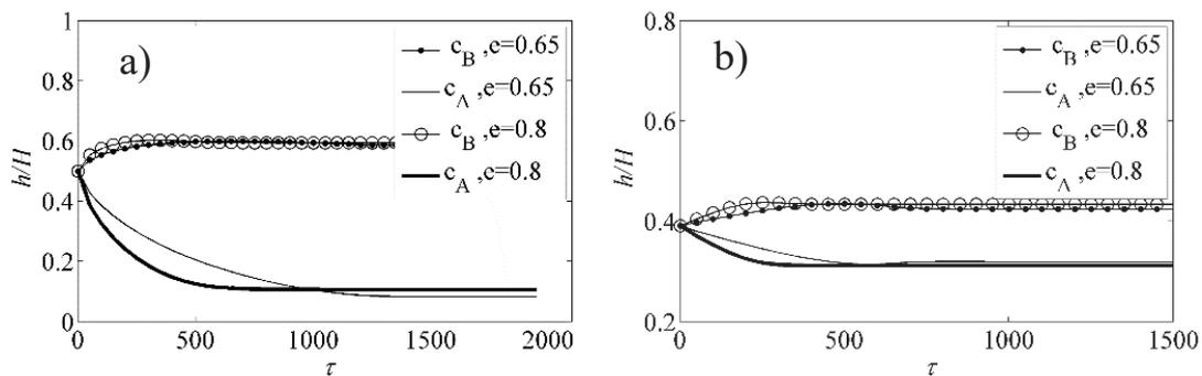
Fig. 6 Time evolution of vertical position of center of mass of area occupied by concentration profile for two fractions and different values of coefficient of restitution for simulation using a) uniform concentration distribution, b) linear concentration distribution
