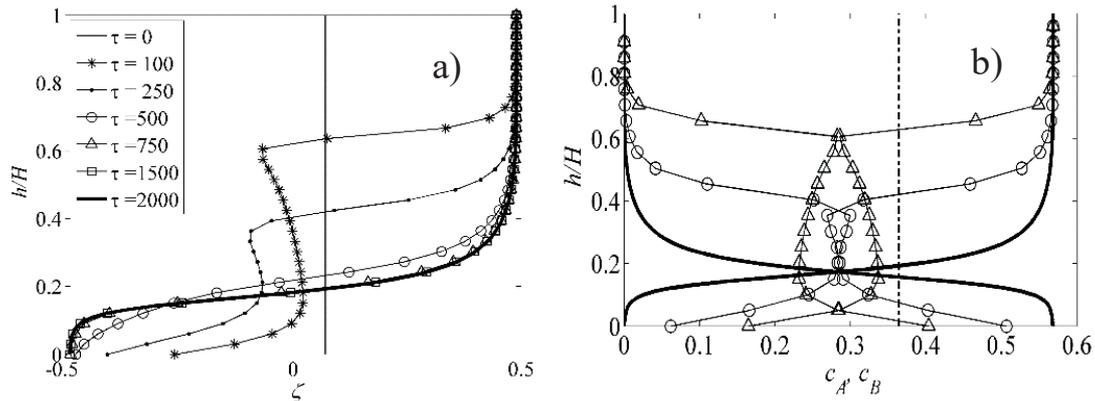
Fig. 4 Time evolution of concentration profiles of both fractions for  $rB = 1.1rA$  and  $e = 0.8$  (typical for plastic grains), Legend: dash dot - initial state ( $\tau = 0$ ), triangle - situation at  $\tau = 500$ , circle  $\tau = 1000$ , thick line  $\tau = 2000$
