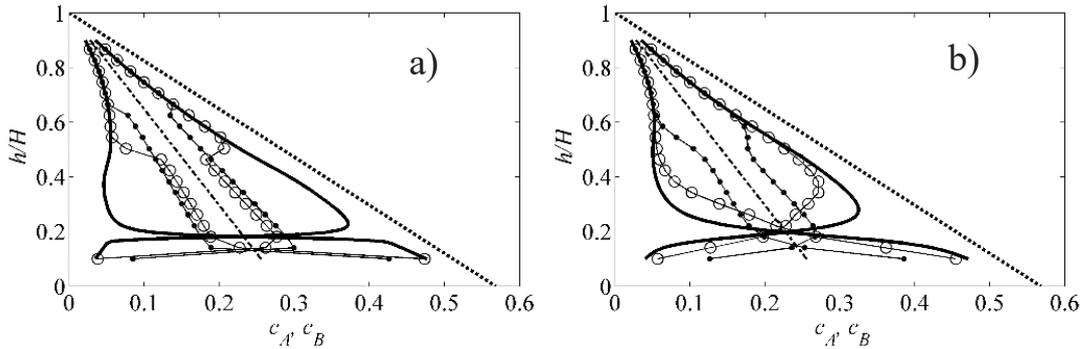
Fig. 5 Time evolution of originally linear concentration profiles of both fractions for  $\Gamma_B = 1.1\Gamma_A$  and a)  $e = 0.65$ , b)  $e = 0.80$ ; dash dot - initial state ( $\tau = 0$ ), line with point- situation at  $\tau = 100$ , line with circle  $\tau = 250$ , thick solid  $\tau = 2000$
