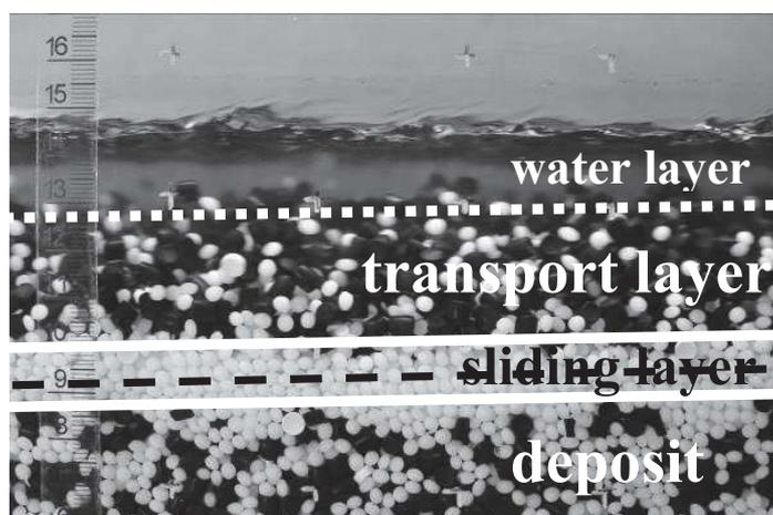
Fig.1 Distribution of grains of sediment fractions in bimodal flow in upper plane bed regime (black – coarser grains, white – finer grains). Legend: white solid lines – boundaries of interfacial sliding layer, black dashed line – top of stationary deposit, white dashed line – top of collisional transport layer
