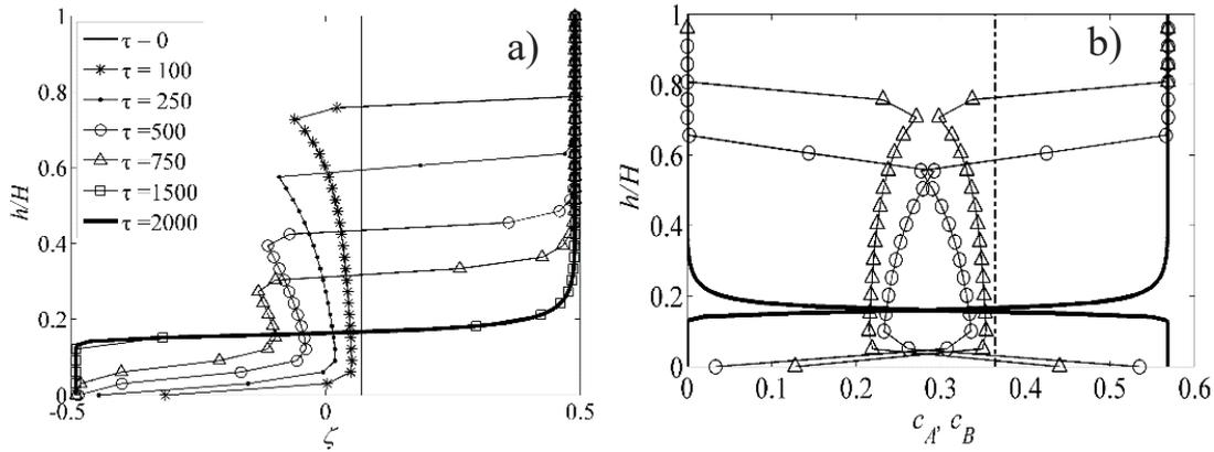
Fig .2 a) Time evolution of dimensionless segregation in uniform concentration profile, b) Time evolution of concentration profile of both fractions due to sorting. Legend: dash dot - initial state ( $\tau = 0$ ), triangle - situation at  $\tau = 500$ , circle  $\tau = 1000$ , thick line  $\tau = 2000$
