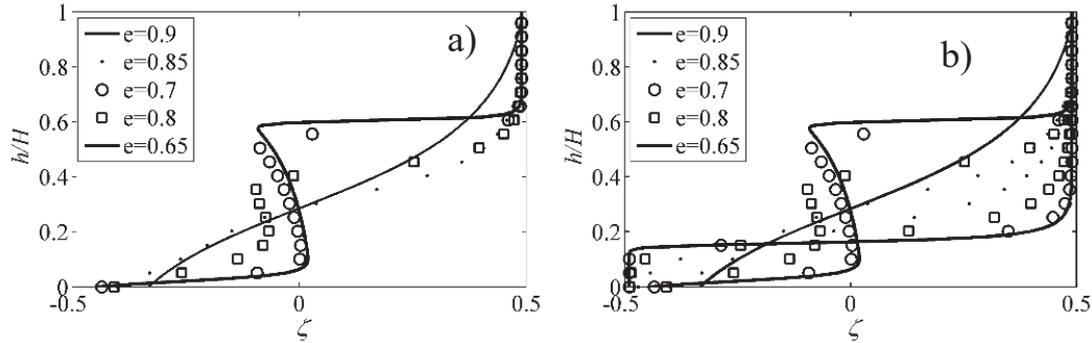
Fig. 3 Sensitivity of dimensionless segregation on coefficient of restitution, a) situation at  $\tau = 250$  (-), b)  $\tau = 2000$  (-)
