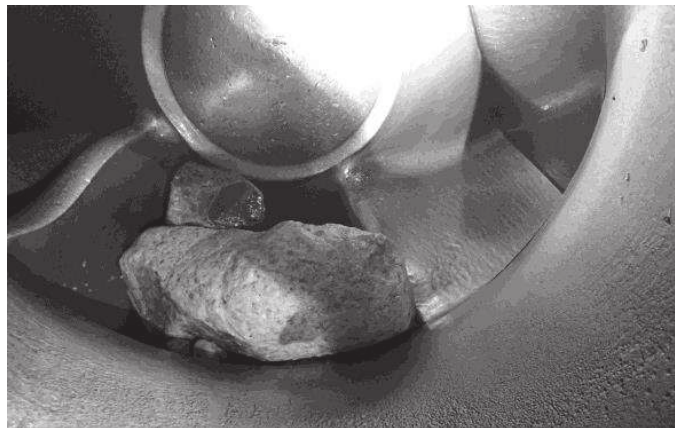
Fig. 13. Dredge pump impeller blocked by stones
