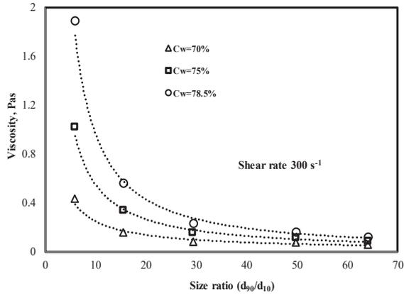
Fig. 2(a) Effect of size ratio ( $\lambda$ ) on viscosity for the five limestone samples
