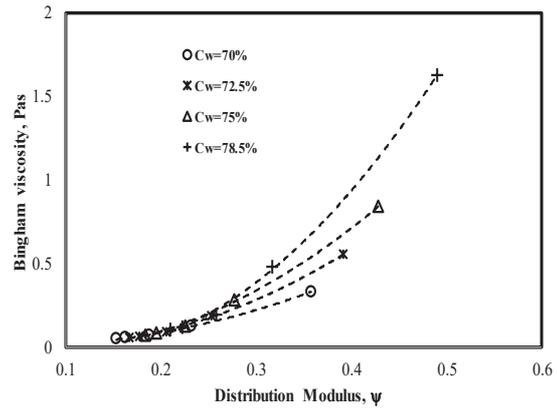
Fig. 2(b) Experimental values of Bingham Viscosity vs. distribution modulus ( $\psi$ ) at different  $C_w$
