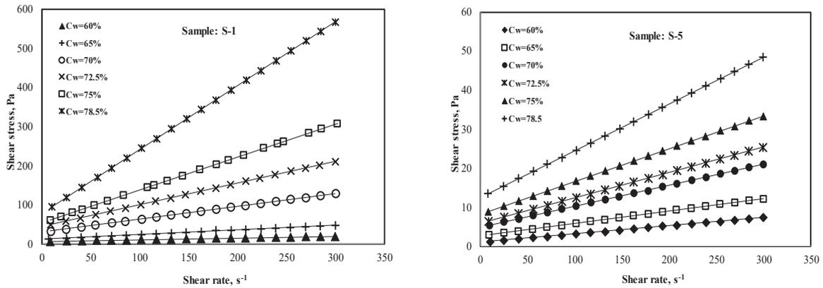
Fig. 1 Rheogram of limestone slurry at different  $C_w$  for sample S-1 & S-5
