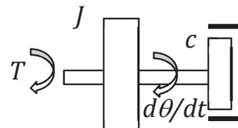
where  $J$  is the polar second moment of mass of the cylinder and  $c$  represents a damping coefficient dependent upon the area of the shearing surfaces.
