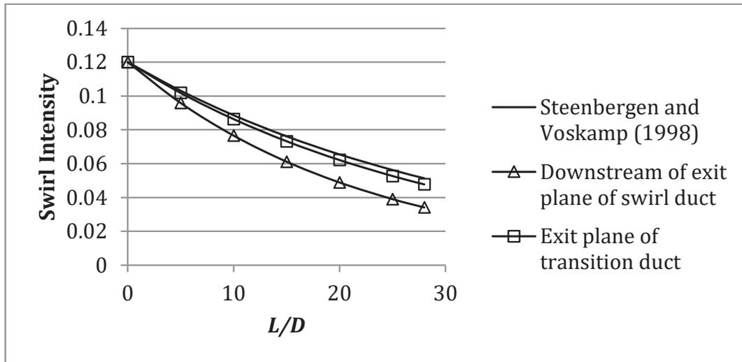
Figure 5: Effect of optimized transition piece after a swirl-inducing duct. The swirl intensity is calculated at the same position with or without the transition duct appended.
