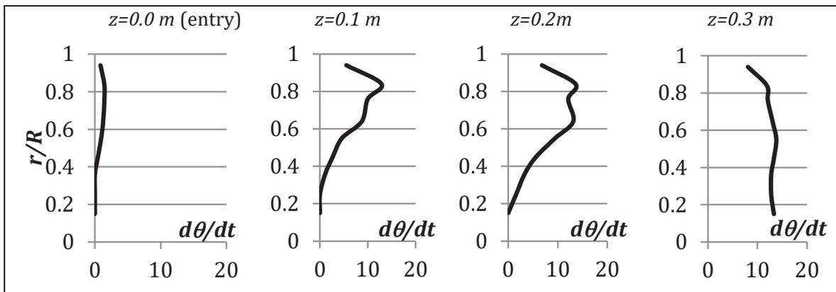
Figure 3: Angular velocity distributions within a 0.4m swirl duct.
