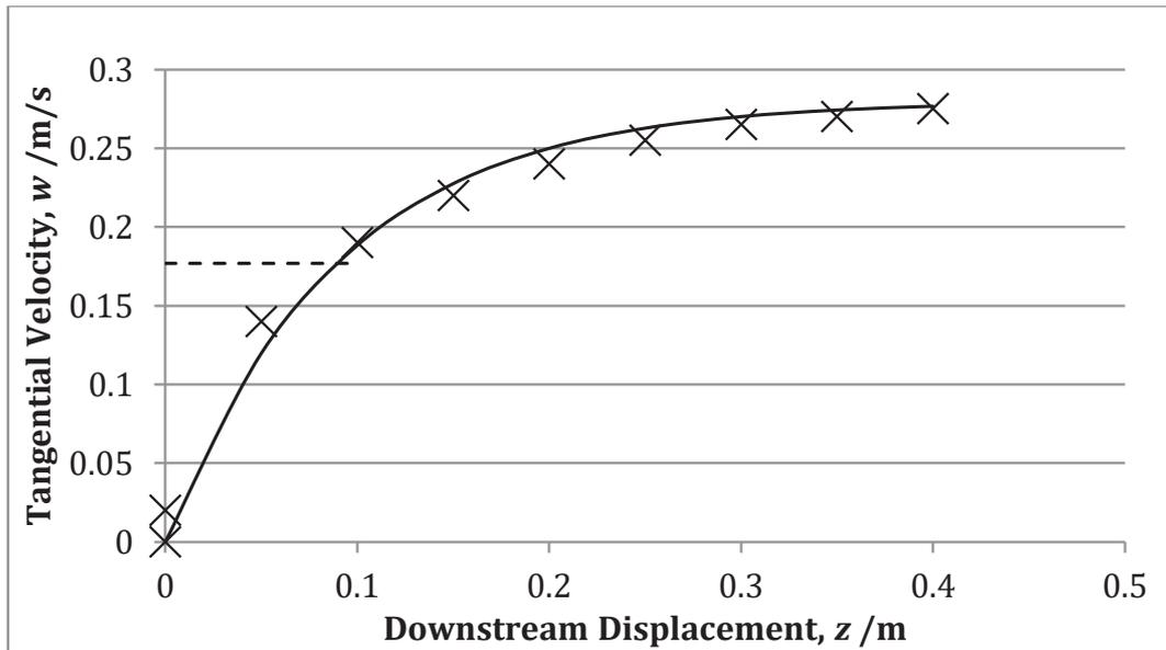
Figure 2: Response of tangential velocity of flow at a fixed radial position in a swirl duct. Axial velocity = 2 m/s. Distance constant  $\tau u \approx 0.1\text{m}$ , so the tangential velocity approaches its maximum 0.28 m/s after 0.3m.
