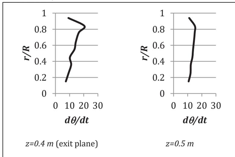
Figure 4: Angular velocity distributions at the exit plane and downstream of a 0.4m swirl-inducing duct.
