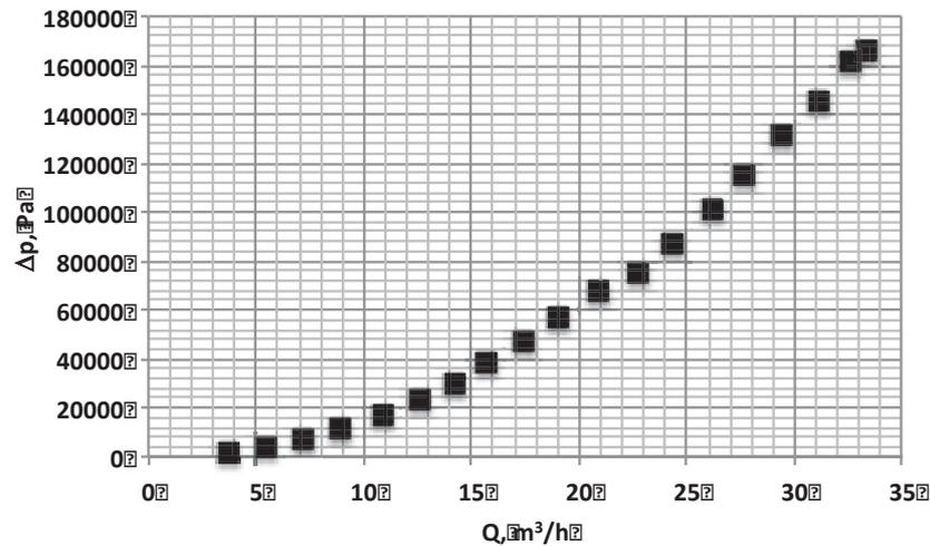
Fig. 4 Measured characteristics of the slotted sieve in a pipeline of inner diameter  $D=0.0545$  m, width of slots  $S=0.00024$  m, open area 16.32%
