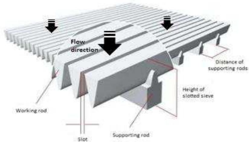
Fig. 2 View of a slotted sieve
