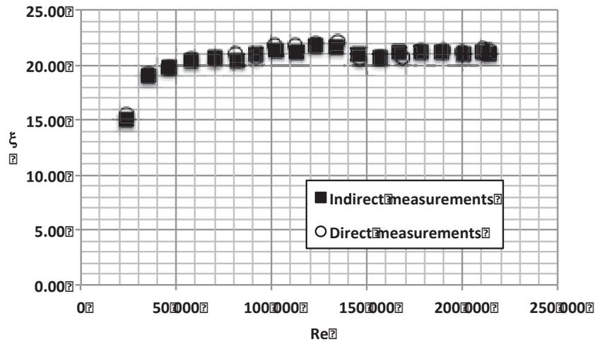
Fig. 5 Experimental data of local frictional coefficient measured using direct and indirect methods in pipeline of inner diameter  $D=0.0545$  m, width of slots  $S=0.00024$  m, open area 16.32%
